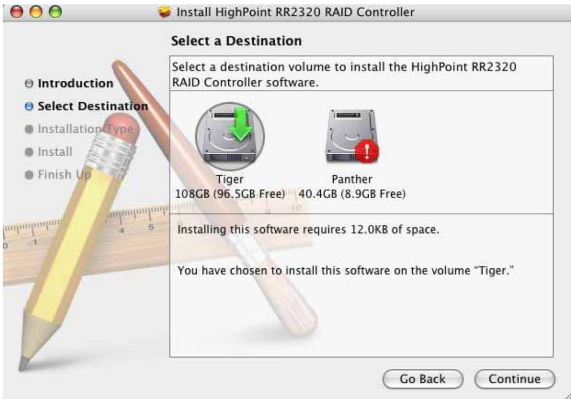
The installer will ask you to select a destination for the driver. Make sure to select the boot volume since the driver has to be installed to /System/Library/Extensions/ folder.
