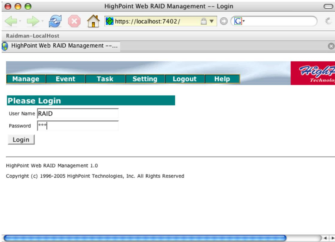
If you can't connect to local system, please check if a process named hptsvr is running on the system. If hptsvr is not running, you can start it manually by running "/Library/StartupItems/Hptsvr/hptsvr".
