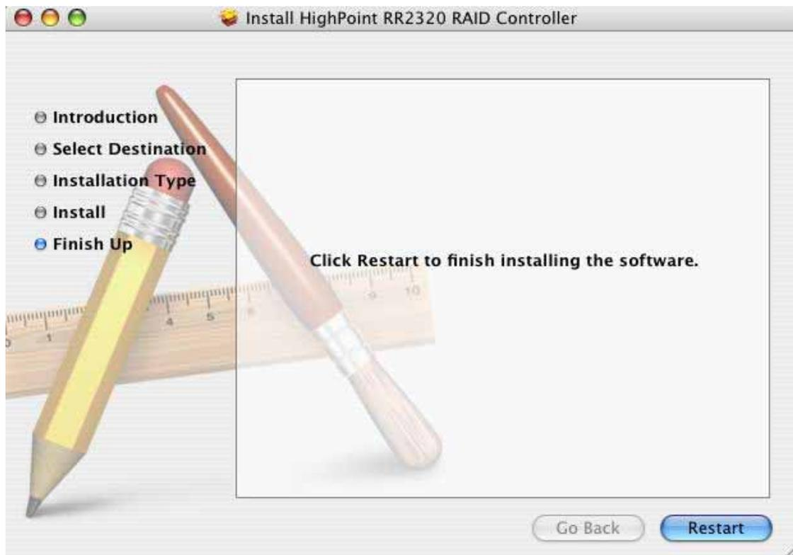
After the system is restarted, you can use a web browser to configure the controller and setup RAID arrays, and use MacOS X Disk Utility to create partitions on the RAID arrays.
