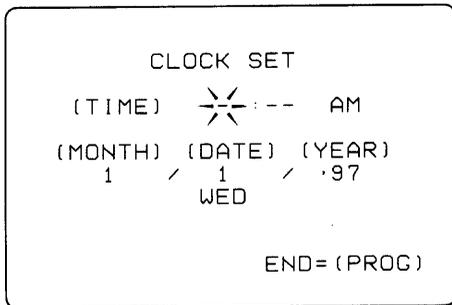
3. Press button **NUMBER "0"** and then "8" to set the hour indication to "8". The minute indication now blinks. If the hour indication is correct, skip this step by pressing the **SHIFT** ← / → buttons.
