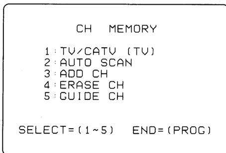
2. Press button **NUMBER 2** to select the AUTO SCAN mode. The indication "AUTO SCAN" blinks on the TV screen and starts scanning all the receivable channel from the lowest channel. When the VCR completes scanning all the receivable channels, the normal TV screen will be restored.
