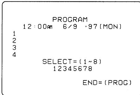
2. Enter the program data with **NUMBER** buttons and press the **SHIFT** ← / → buttons to skip steps that do not require adjustments.
