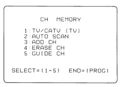
Each time you press button NUMBER 1, the display changes between TV/CATV (TV) and TV/CATV (CATV).
