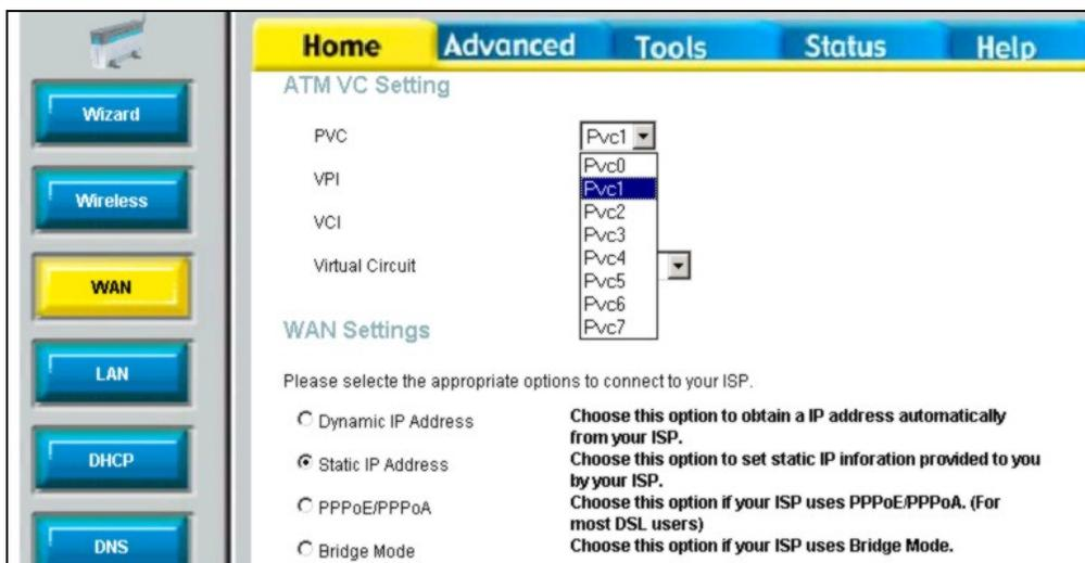
Figure 4- 20. Select new PVC to configure in the WAN menu
