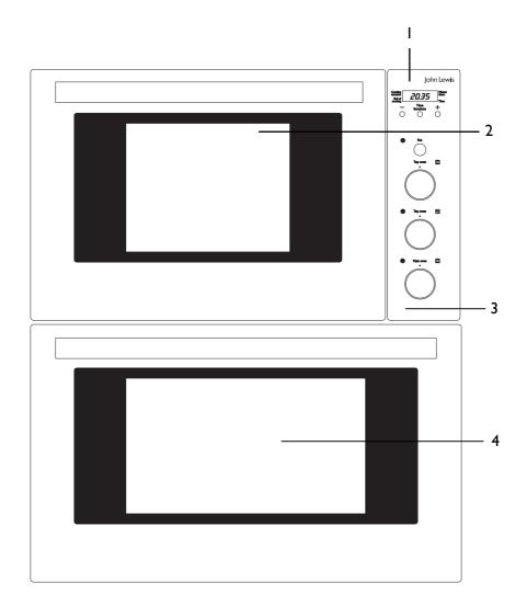
Your built-under appliance comprises of a conventional oven and dual grill in the top compartment. The main fan oven can be automatically controlled by the electronic timer.
