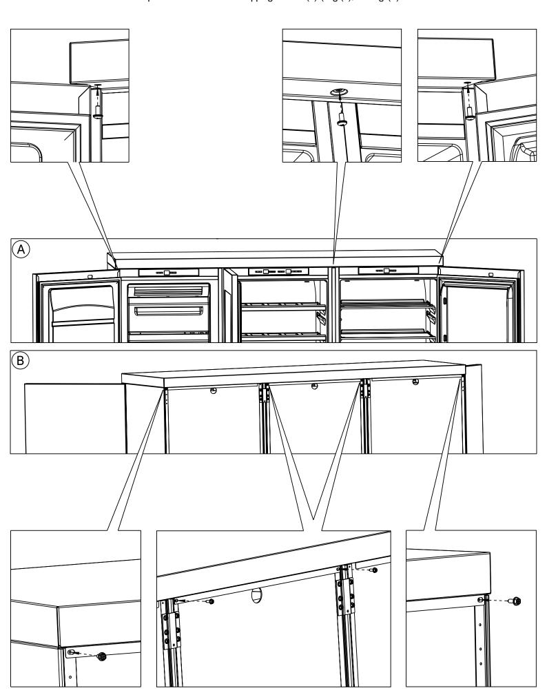
• Fit the trims "II" between the units (freezer/wine cooler - wine cooler/cooler) by pressing along the entire profiles, see figure below.
