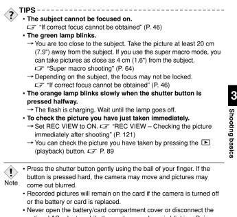
Never open the battery/card compartment cover or disconnect the optional AC adapter while the card access lamp is blinking. Doing so could destroy stored pictures and prevent storage of pictures you have just taken.
