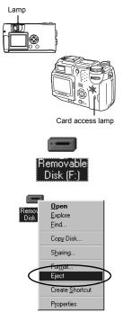
4 Make sure that the lamp on the right of the viewfinder or the self-timer lamp (which on some models light while the camera is connected to the computer) or the card access lamp is not blinking.
